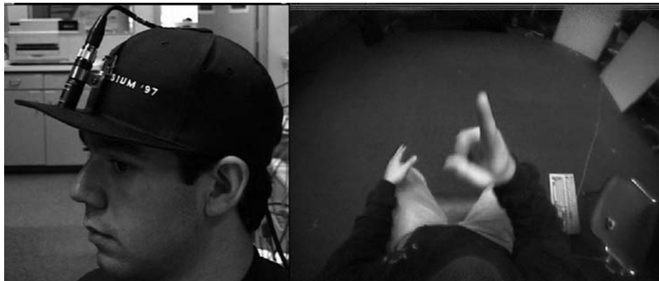
FIGURE 38.3 A sign recognition system using a hat-mounted camera that obtains an overhead image of the signer's hands. (From Brashear, H., Starner, T., Lukowicz, P., and Junker, H., Using multiple sensors for mobile sign language recognition, in the Proceedings of the 7th IEEE International Symposium on Wearable Computers , 21–23 October 2003, White Plains, NY, pp. 45–52, Elsevier, IEEE, 2003.)
