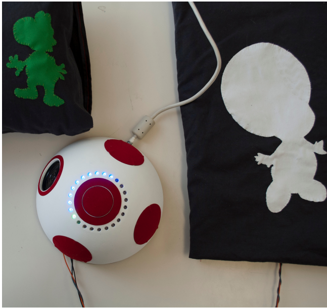
Figure 2. The Rattle Alarm System – Developed together with Mia – left: cushion, middle: alarm clock, right: pressure mat
