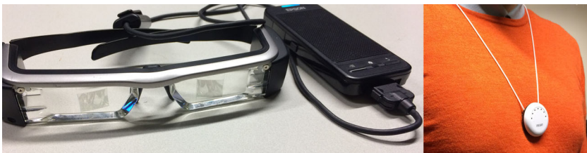
Figure 5. Left: The EPSON BT-200 HMD shown with its touchpad controller that participants wore to access the Digital Selves. Right: The MeCam Classic wearable camera that participants wore to record interactions
