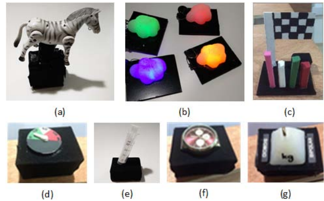
Figure 2. Active tangible objects contextualized for ANN operations including; a) Horse - Context Simulator Controller, b) Clouds – Hidden Layer nodes, c) Finish Podium – Output Visualization, d) Speedometer – Input Speed Value, e) Syringe – Input Health Value, f) Chronograph – Output Time Value, g) Weight – Synapse Weight Adjustment.
